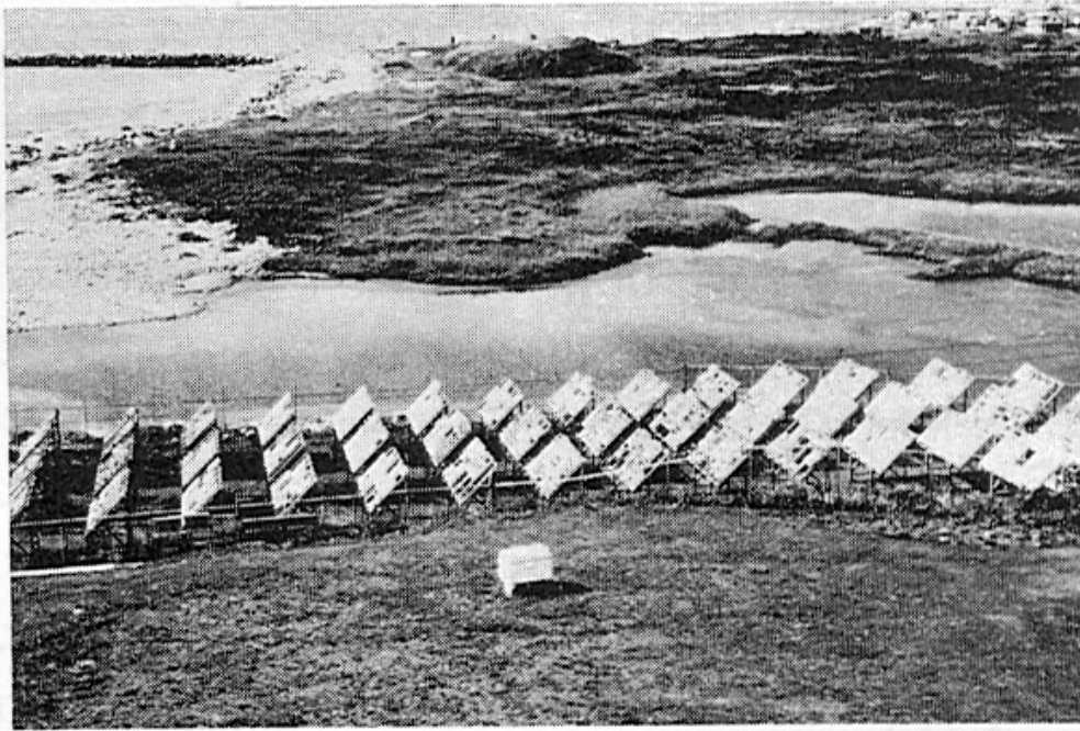
FIGURE 15-4 — Atmospheric test station in Rhode Island for exposure of specimens to atmosphere representative of Northeastern U.S. seacoast.
